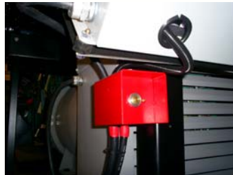
Battery box and batteries are mounted inside the main frame rails with the cutoff switch mounted on the pedestal and below the control panel.
