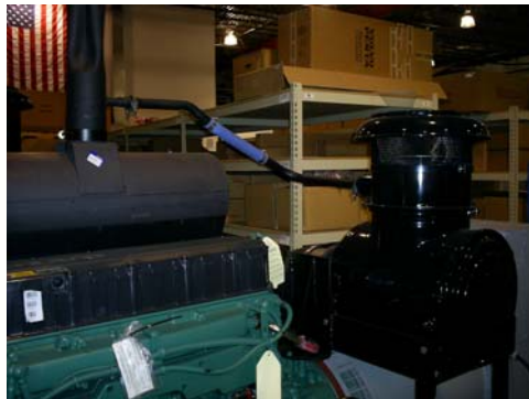
Two stage Donaldson air cleaner for dusty environments with heavy particle exhaust ejector. Muffler assembly is mounted on the skid frame for easy assembly into a trailer
